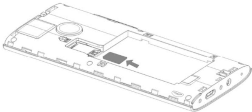
**An SD memory card can be pushed in above the SIM card.**
