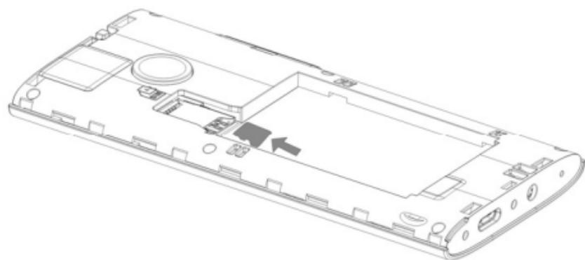
**The battery is inserted next (this is only possible in the correct position).**
